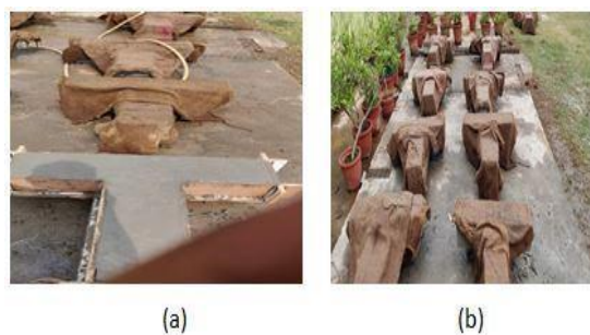
Figure 3: (a) Casted specimens, (b) Curing of specimens
