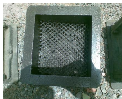
Figure 4: Image showing the Geosynthetic material added to beam and cube
